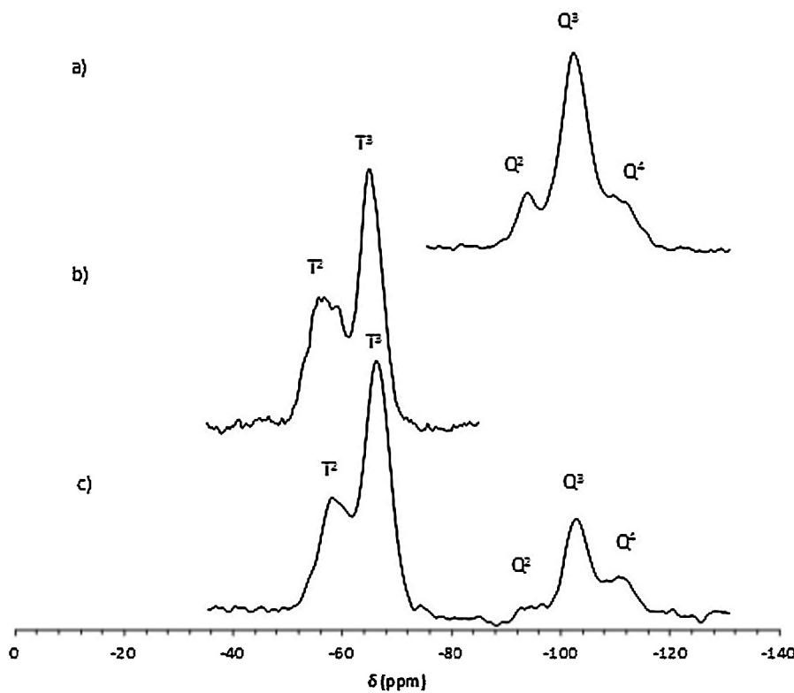
**Fig. 1.**  $^{29}\text{Si}$  solid NMR spectra of (a) TEOS, (b) MTMOS, and (c) MTMOS:TEOS molar ratio 7:3.
