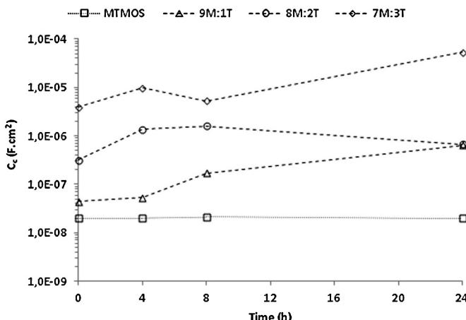
**Fig. 8.** Evolution of the coating capacitance versus time of contact with electrolyte of the coatings MTMOS, 9M:1T, 8M:2T and 7M:3T.
