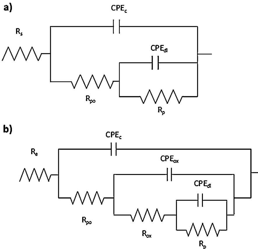
Fig. 4. Equivalent circuit a two time constants and b three time constants.
