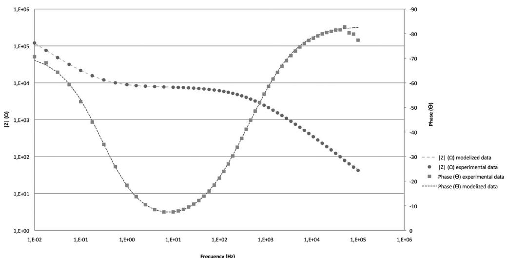
Fig. 6. Bode plot for 8M:2T sample after 10 h in contact with electrolyte. Comparison between experimental data and modelisation results with equivalent circuit.
