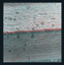
SEM microphotographs of the PHOENIX implant. Surface roughness with craters
