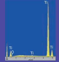
Results of microanalysis using the energy dispersal X-ray (EDS) of the surface of an llerimplant implant. **Titanium oxide**.
